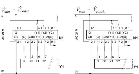
Modulating control  $\dot{V}_{max}$  and  $\dot{V}_{min}$  and complete shutoff and fully open operating mode "con"
