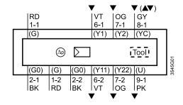
Tool = Configuration and maintenance interface (Series E: 7-pin)
